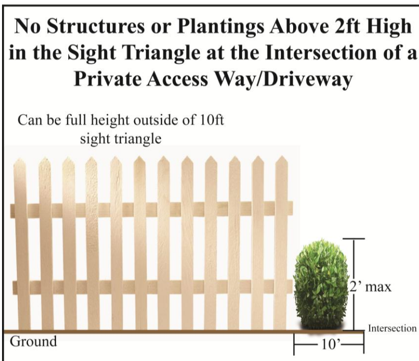
Figure 4: Height Restrictions in the Sight Triangle at a Driveway
